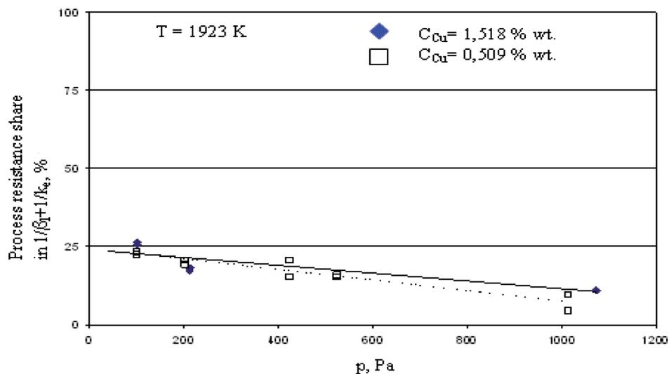
Fig. 3. Share of total resistance in the liquid phase and the evaporation process resistance in the total copper evaporation resistance (for the tests conducted at  $p > 100$  Pa)
