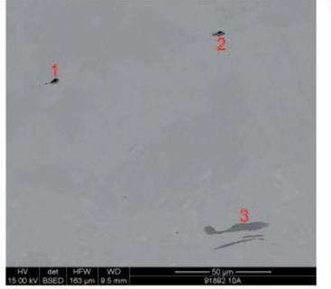
Fig. 2. Characteristic non-metallic inclusions in the sample of rolled bar ( $\emptyset$  50 mm) from melt no. 91892 (LF, VD) ladle treatment duration 100 min, II series, magnification 1000x
