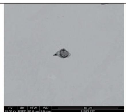
Fig. 3. Characteristic non-metallic inclusions in the sample of rolled bar ( $\varnothing$  50 mm) from melt no. 91893 (LF) ladle treatment duration 190 min, II series of tests, magnification: 1000x
