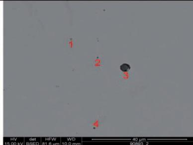
Fig. 1. Characteristic non-metallic inclusions in TOS sample from melt no. 90893 (end of secondary treatment), ladle treatment duration 190 min, I series, magnification 1000x
