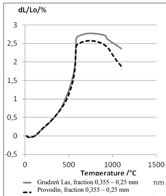
Fig. 2. Thermal expansion of silica sand
