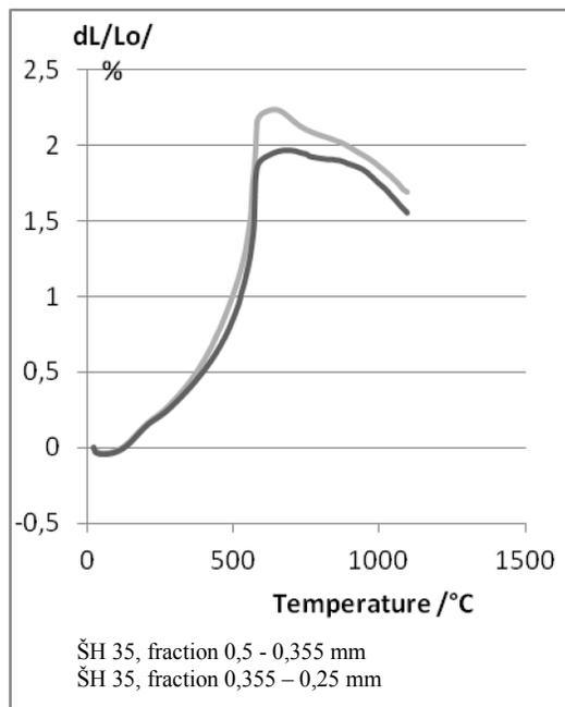
Fig. 1. Thermal expansion of sand ŠH 35
