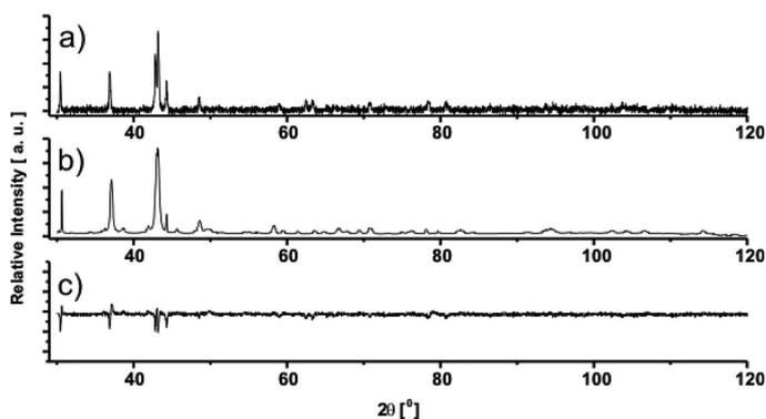
Fig. 3. X-ray diffraction patterns obtained for  $\text{Sm}_{12.5}\text{Co}_{66.5}\text{Fe}_8\text{Cu}_{11}\text{Si}_2$  alloy, obtained using a wheel linear velocity of 20 m/s: a) measured, b) calculated from the Rietveld analysis, c) difference between measured and calculated results
