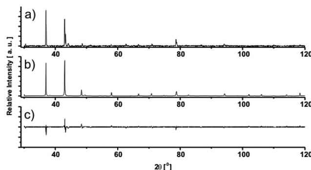
Fig. 2. X-ray diffraction patterns obtained for  $\text{Sm}_{12.5}\text{Co}_{66.5}\text{Fe}_8\text{Cu}_{11}\text{Si}_2$  alloy, obtained using a wheel linear velocity of 18 m/s: a) measured, b) calculated from the Rietveld analysis, c) difference between measured and calculated results
