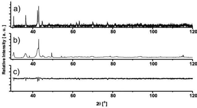
Fig. 4. X-ray diffraction patterns obtained for  $Sm_{12.5}Co_{66.5}Fe_8Cu_{11}Si_2$  alloy, obtained using a wheel linear velocity of 22 m/s: a) measured, b) calculated from the Rietveld analysis, c) difference between measured and calculated results
