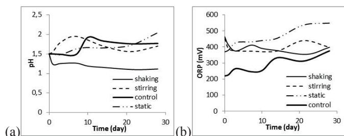
Fig. 2. (a) The pH changes over the leaching time, (b) Changes in oxidation-reduction potential during bioleaching study.
