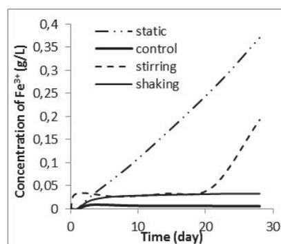
Fig. 3. Changes of  $\text{Fe}^{3+}$  concentration with time on leaching PCBs.
