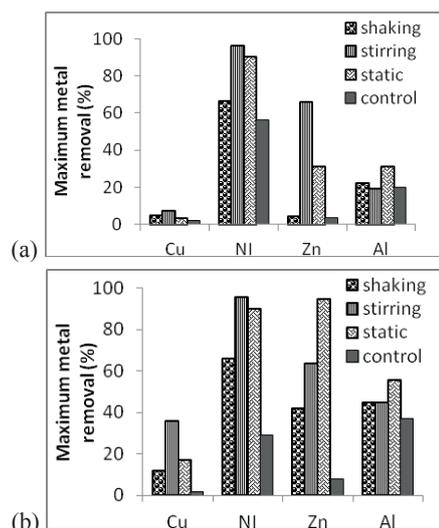
Fig. 4. The percentage of copper, nickel, zinc and aluminium solubilized from PCBs: (a) calculated for the 14<sup>th</sup> day, (b) at the end of the process.
