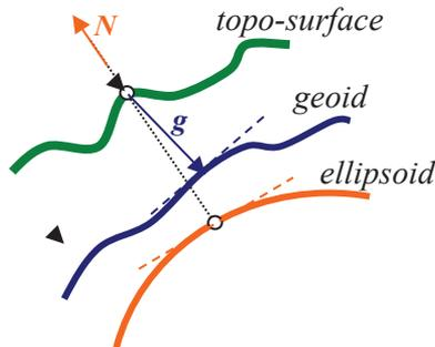
Fig. 5. The normal vector of the ellipsoid and the vector of gravity
