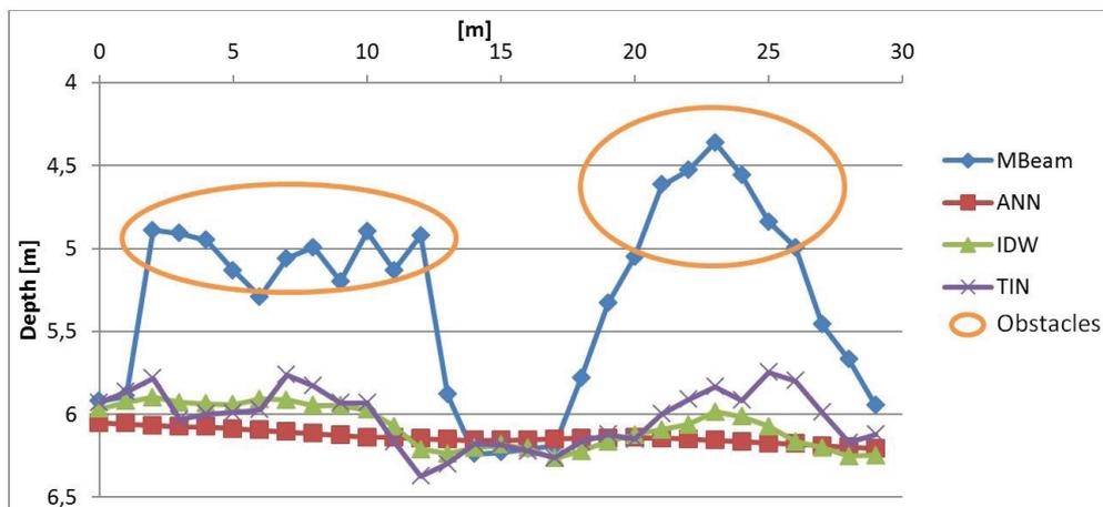
Fig. 4. Profile CS-1 of DTMs obtained by all methods showing the underwater obstacles based on the interpolation of 100% of the points. MBeam- multibeam data, ANN- Artificial neural network, IDW- Inverse Distance Weighting, TIN- Delaunay Triangulation
