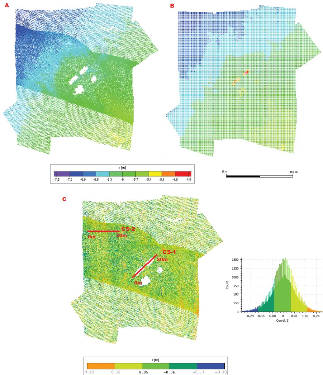
Fig. 3. A) Airborne laser bathymetry point cloud of the sea bed;
