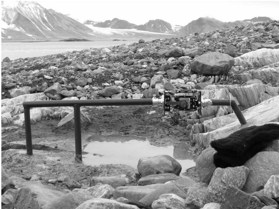
Fig. 1. The TM-71 optical-mechanical crack gauge located in front of the Hansbreen Glacier at Site 1 (Photo by T. Nýdl). The monitored fault  $82^{\circ}/225^{\circ}$  crosses the outcrop beneath the instrument.
